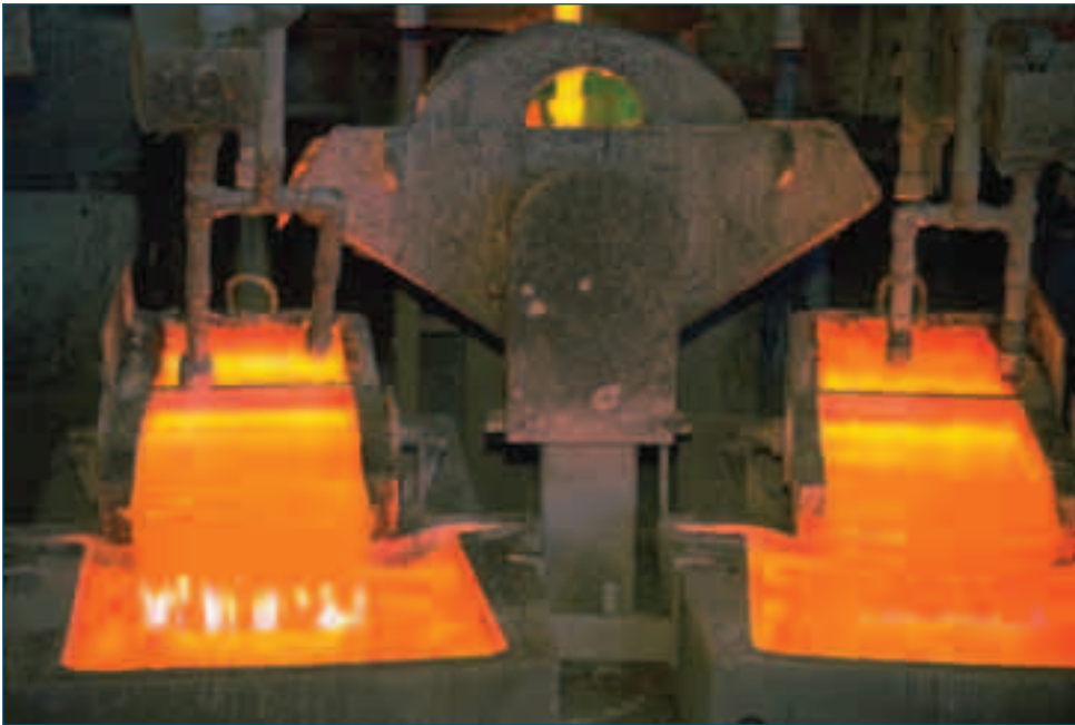
Hot property – copper anodes being poured at MIM's Copper Smelter.
