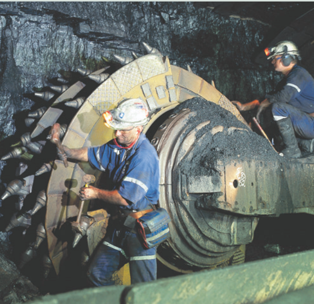
◀ Nigel Wilson, Longwall Maintenance Crew Miner, and Steve Clarkson (PC), Longwall Maintenance Crew Fitter, change picks on the shearer drums at the Newlands longwall.
